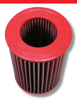
The panel / cylindrical air filter is commonly referred to as "replacement air filter". It is installed in the vehicle's original airbox to replace the OEM air filter. It is made of highly performing materials that allow an increased air flow combined with a more efficient filtration, guaranteeing containment of all impurities from as small as 7 microns (compared to OEM's 10 microns).
