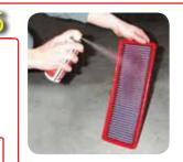
The oiling procedure using the aerosol spray. Hold the spray 15 cm from the filter and spray the complete surface. Repeat the operation on both sides of the filter.
