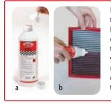
Remove the original top from the regenerating fluid bottle. Make a small hole in the spout dispenser and screw onto the bottle. For correct oiling we recommend passing the regenerating fluid twice over every pleat on both sides of the filter.
