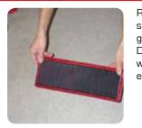
Remove the larger dirt by shaking or tapping your filter gently onto a clean surface. DO NOT use compressed air which may damage the filtering element.
