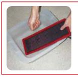
Wash your filter in cold water. Rinse well ensuring that dirt does not enter the filter pleats. DO NOT use high-pressure water.
